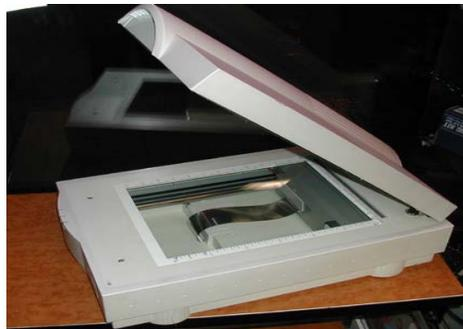
An **A4 scanner** has an affordable price tag and is extremely useful once one has got the right touch. In combination with Optical Character Reading (OCR) software it will save a lot of time when large amounts of paper data need to be put into digital format.
